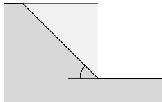
→ **The thrust is due to the sliding wedge**
