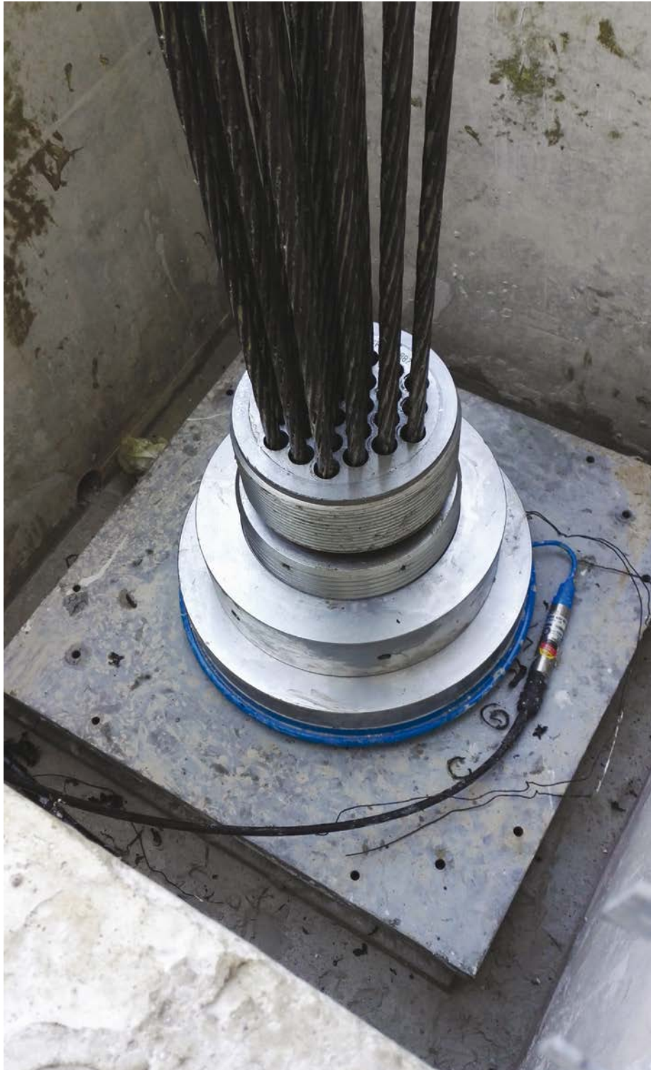
Picture 8.9: Adjustable anchor head with a removable load cell (© Alexis Piron-EDF)
