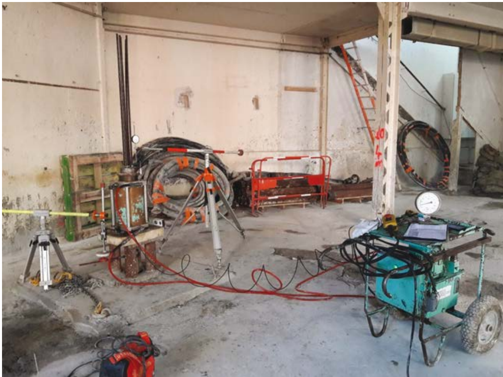
Picture 8.2: example of a failure test system (© Spie Fondations)
