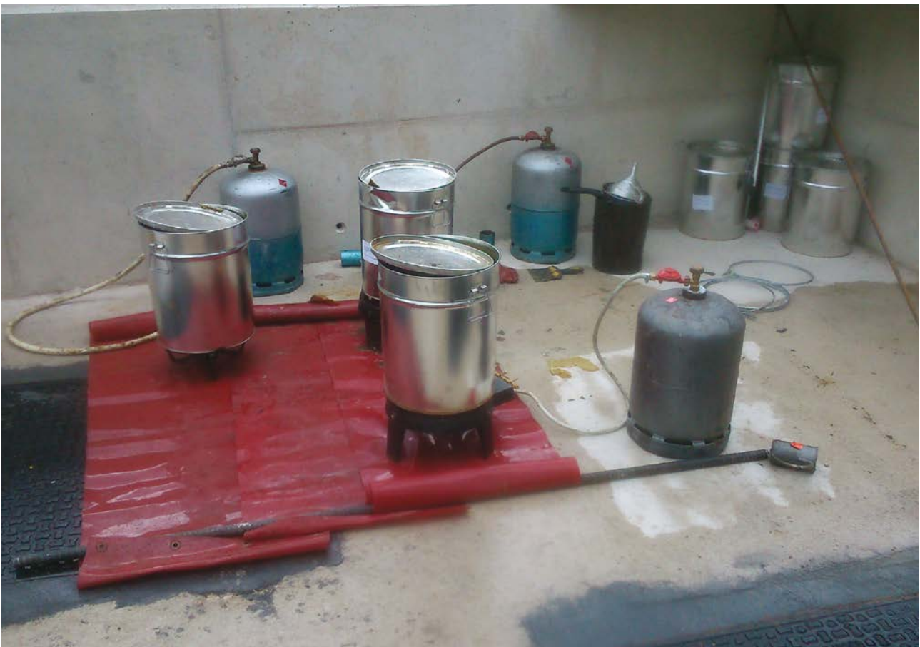
Picture 6.7: Preparation of petroleum wax (anti-corrosion product) (© Alexis Piron-EDF)
