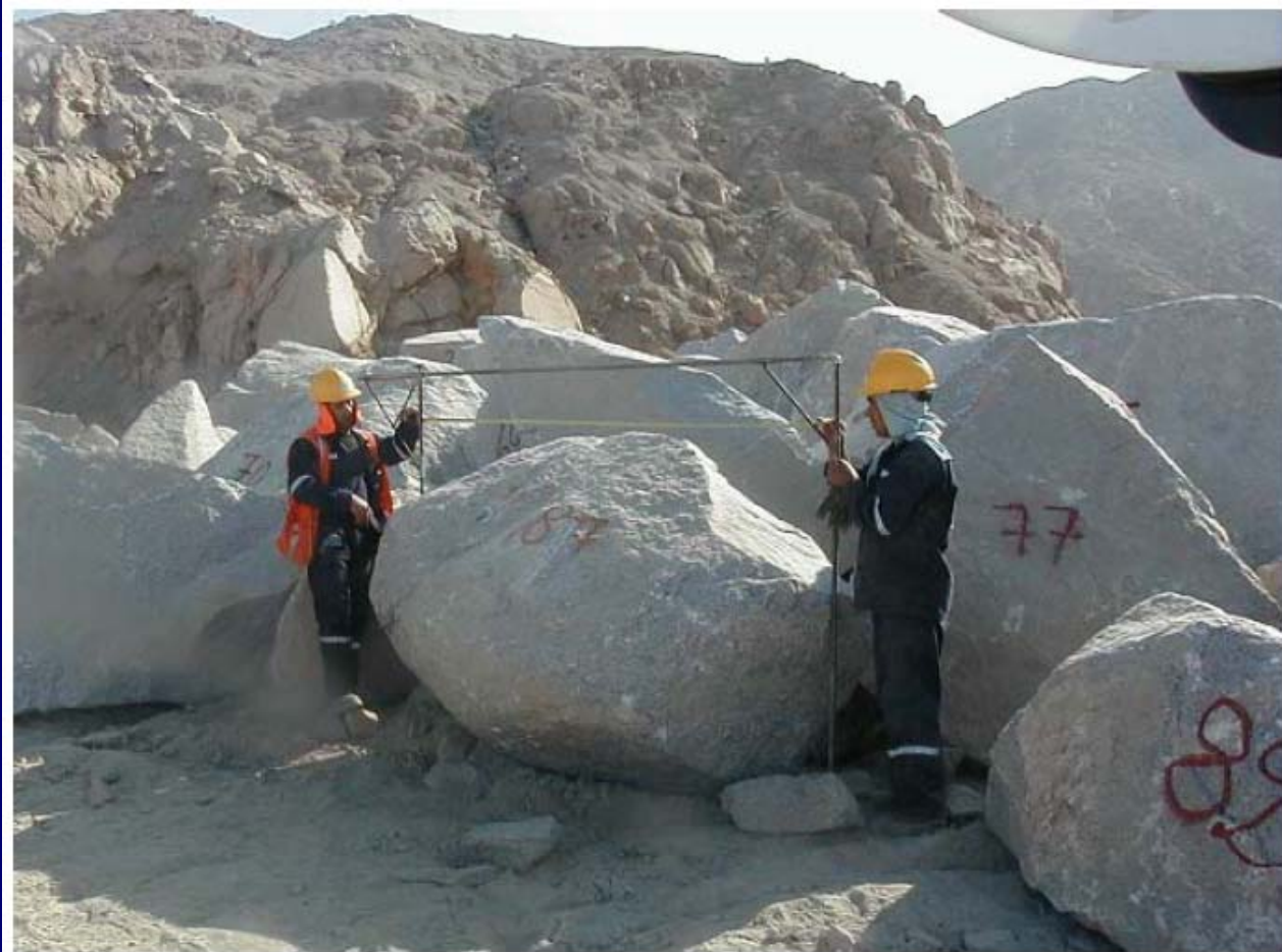
Figure 6: Measuring rocks with a simple vernier.
