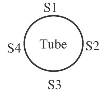
Soil pressure cells on the pipe
