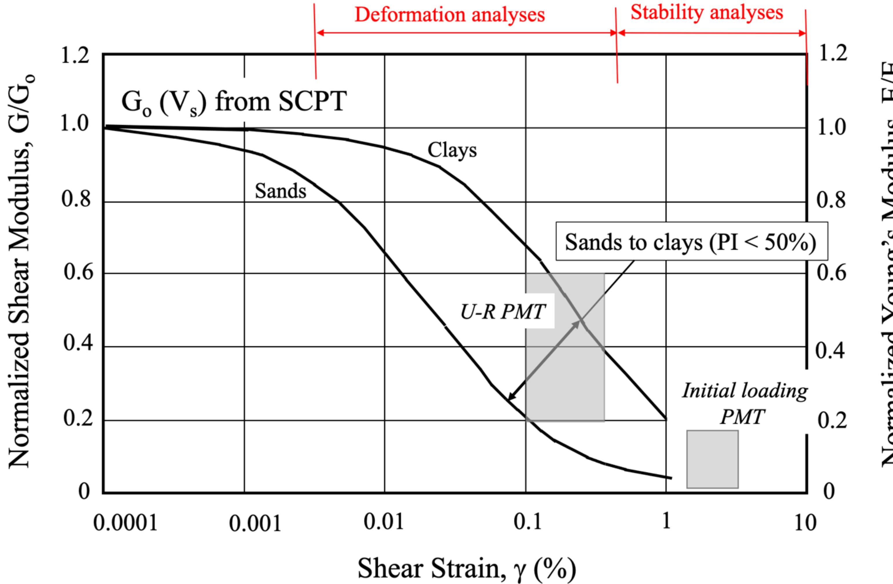
Measure  $V_s$  (small strain) to get  $G_o (E_o)$  and unload-reload Modulus ( $E_{UR}$ ) from PMT to evaluate modulus degradation curve with strain
