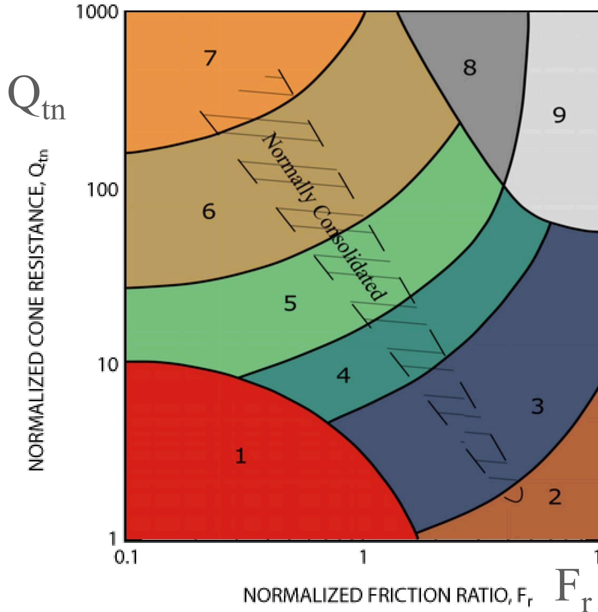
CPT SBT based on in-situ soil *behavior* - not the same as traditional classification based on *physical* characteristics using Atterberg Limits and grain size carried out on disturbed samples
