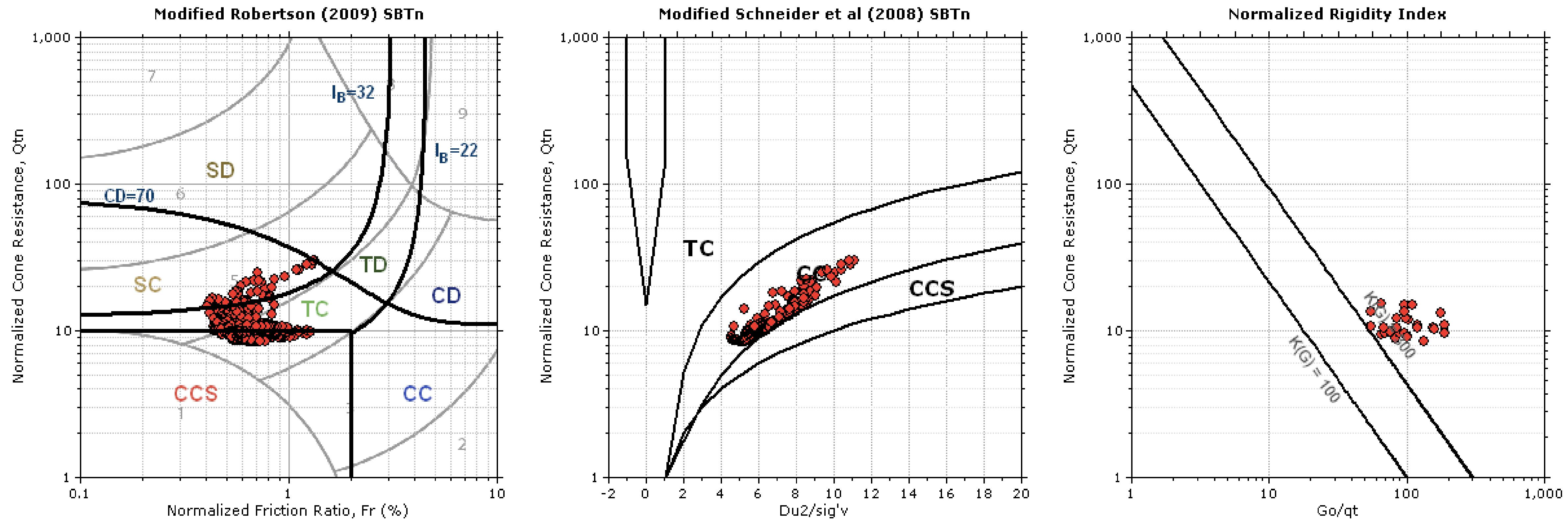
SCPTu data from 20 to 50m in Cooper Marl (calcareous cemented clay/silt),
