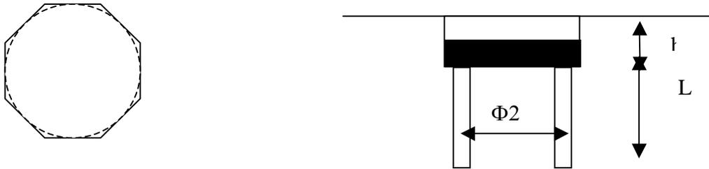
**Figure 15: Diagram of a pile-raft foundation.**
