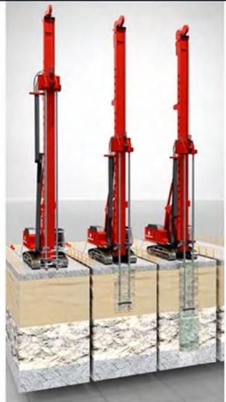
Double Auger Soil Mixing technique
