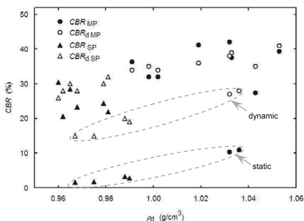
Figure 3. Relationship between  $CBR$  value and dry density with an indication the points obtained at moisture contents at compaction  $w=w_{opt}+(2.5-5\%)$ : MP – Modified Proctor method, SP – Standard Proctor method,  $CBR$  – static test results,  $CBR_d$  – dynamic test results.
