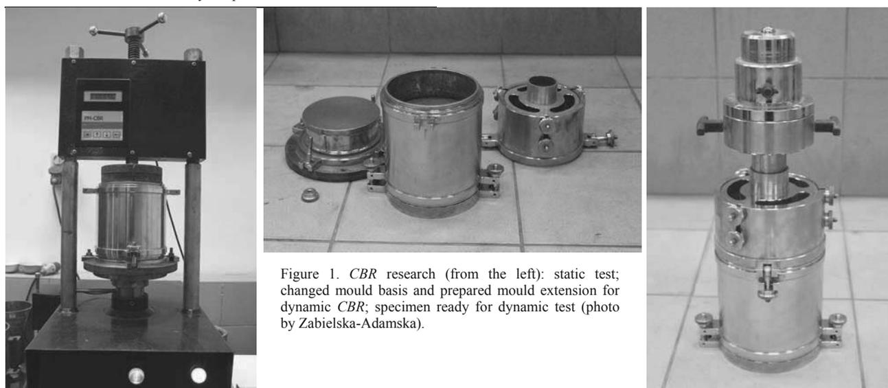
Figure 1. *CBR* research (from the left): static test; changed mould basis and prepared mould extension for dynamic *CBR*; specimen ready for dynamic test (photo by Zabielska-Adamska).
