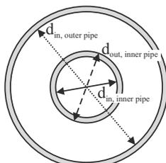
Figure 2. Freeze pipe diameters to calculate hydraulic diameter.
