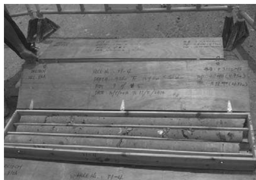
Figure 6. Typical core sample obtained from jet grout column
