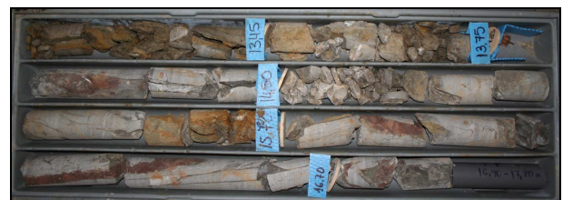
Figure 3. Drill cores from a borehole in Zone 3.
