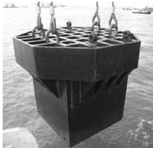
Figure 10. Specially designed multi-purpose marine pounder (Chu et al., 2009)
