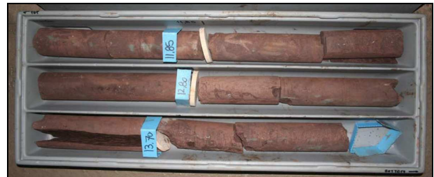
Figure 2. Drill cores from a borehole in Zone 2.
