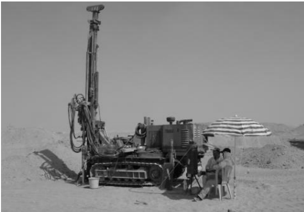
Figure 4. Pressuremeter testing at Al Qu'a new township
