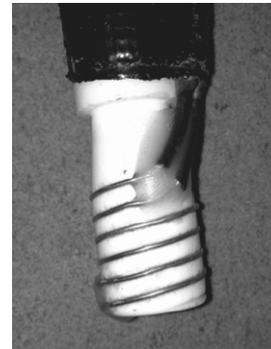
Figure 4. Coiled TDR constructed around a ceramic tensiometer body
