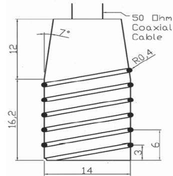
Figure 3. Schematic of tensiometer housing and coiled TDR (dimensions in mm)
