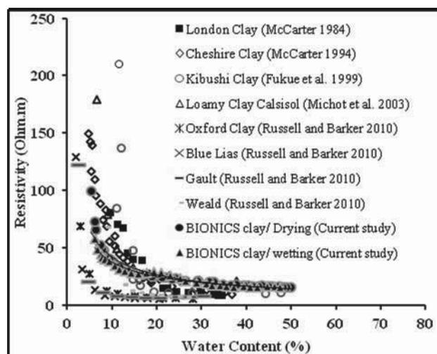
Figure 2. Resistivity-water content relationships of BIONICS clay and different clays reported in the literature
