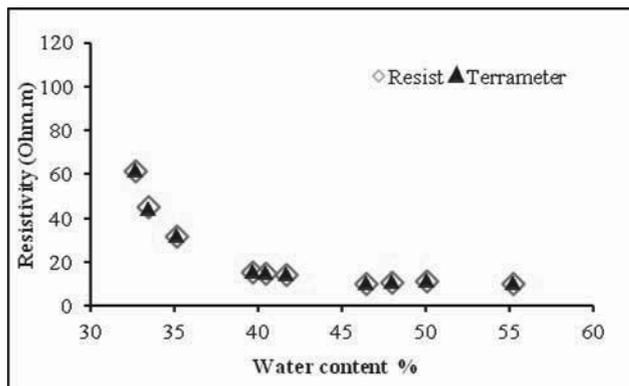
Figure 1. Resistivity-gravimetric water content relationship of a kaolin specimen
