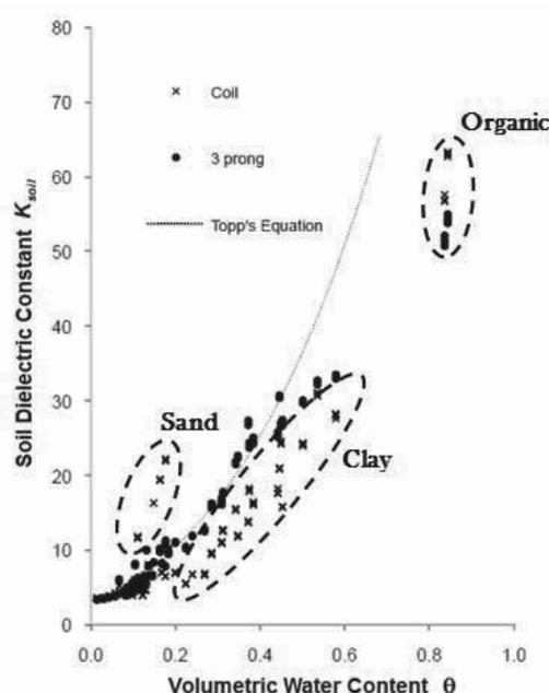
Figure 5. Comparison between the Coiled TDR (with a steel tensiometer housing) and a conventional 3 prong TDR device for Leighton Buzzard sand, Birtley Clay and a very loose organic soil.
