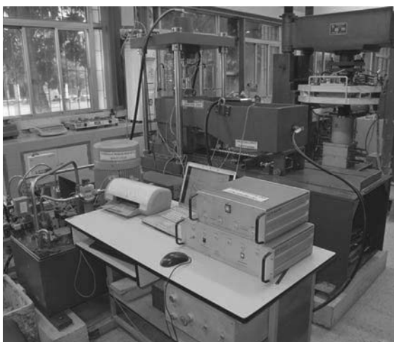
Figure 2 Close up view of large scale direct shear machine (Rao and Shrivastava 2009).
