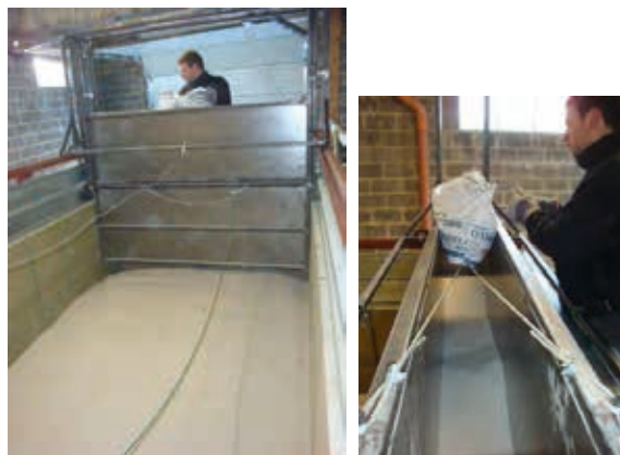
Figure 1. The sand deposition by the pluviation technique.
