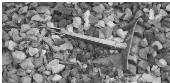
Figure 12. Position of anchor at the end of an 80-g test.
