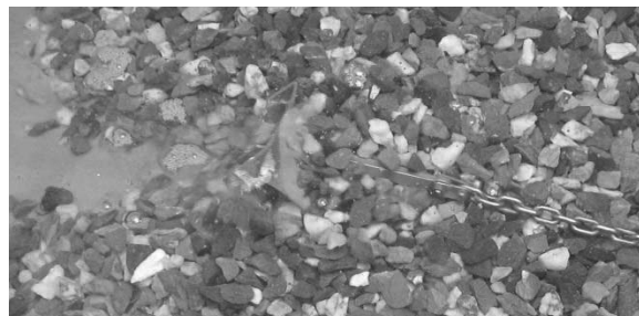
Figure 13. Position of anchor at the end of last 1-g test.
