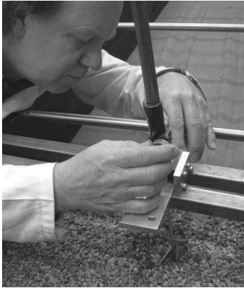
Figure 7. Carefully measuring the position of the anchor after a test.
