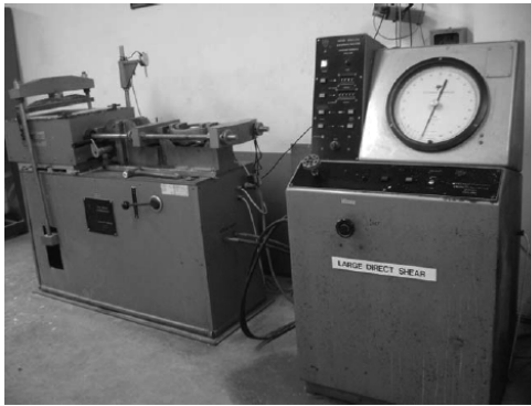
Figure 6. Large scale direct shear apparatus (Artidteang et al., 2012)
