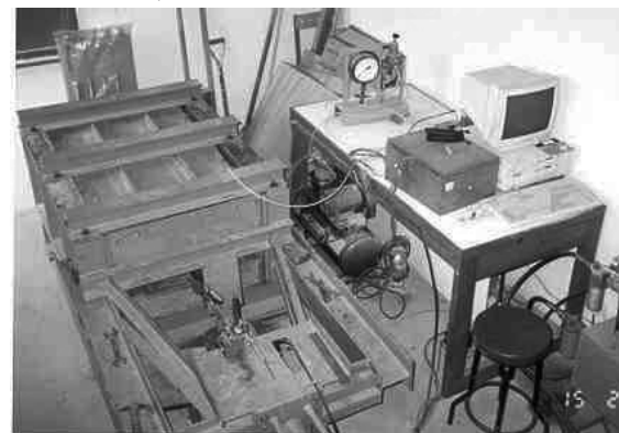
Figure 3. Pullout machine (Artidteang et al., 2012)
