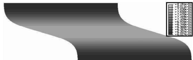
Figure 4. Deformed configuration of granular layer under P_0 = 100 \text{ kPa} after U_{1B} = 1.5 h_0 along with contour plot of void ratio ( e_0 = 0.6 , d_{50} = 1 \text{ mm} ).
