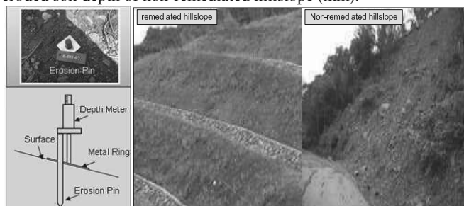
Figure 5. Schematic layout and photos of erosion pins embedded in remediated/non-remediated hillslope.
