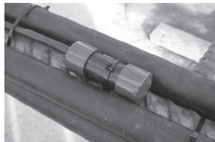
Figure 2. Base of the central thermistor string prior to installation of the U-tubes and steel bar.
