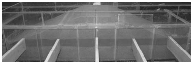
Figure 9. Small-scale model test of a flood protection dyke with simulated subgrade (fine-grained cover layer and permeable aquifer).
