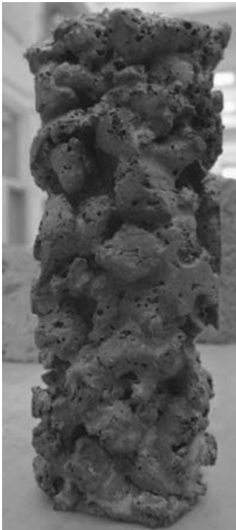
Figure 3. Cement, sand and glass foam mixture sample for the unconfined compression test (Tuncel, 2012).
