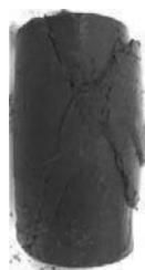
Photograph 1 Failure shape of the test specimen
