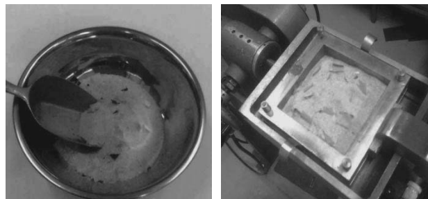
Figure 2: a) Soil-plastic composite b) Composite specimen placed in shear box for testing
