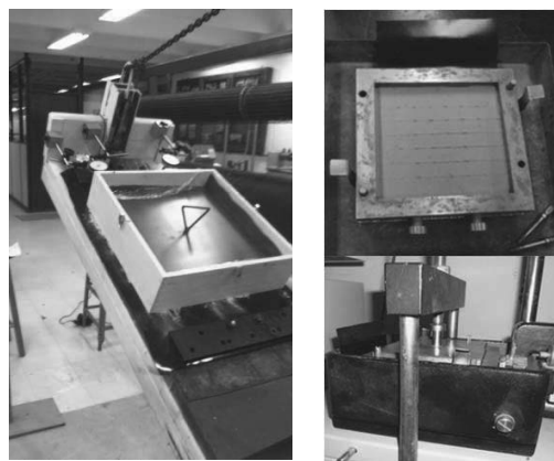
Figure 2. (a) Ramp test and (b) Conventional direct shear test.
