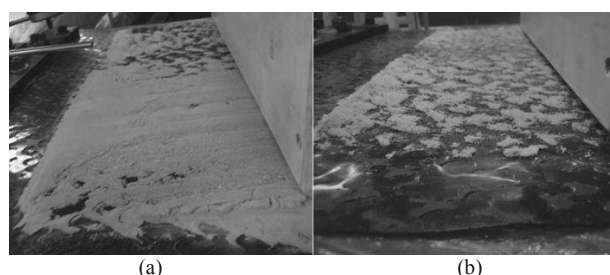
Figure 5. Tests on texturized HDPE geomembrane: (a) degree of saturation of 5.5% and (b) degree of saturation of 66%.
