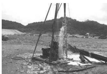
Figure 4 . Ejection of leachate/gas (Chen et al., 2013)
