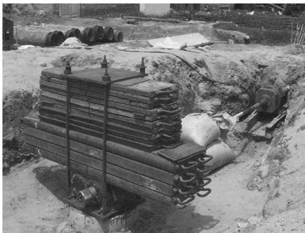
Figure. 1 Complete setup of vertical vibration test on full-scale pile
