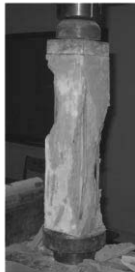
Figure 2. Axial compression testing of test samples
