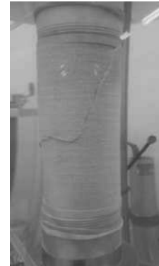
Photo 2. Condition of the test specimen after shear
