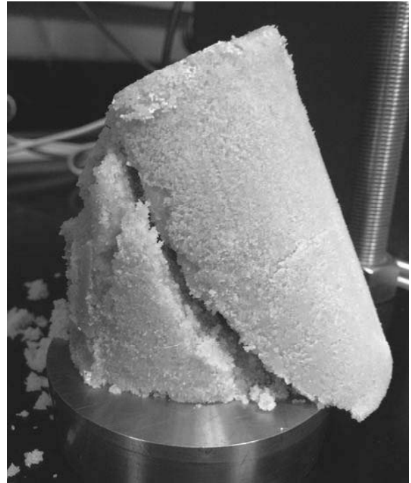
Figure 5. Failed cemented soil column at the end of the unconfined compression test.
