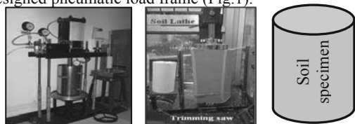
Slurry consolidation Specimen trimming Final specimen size Figure 1. Consolidation set-up on the laboratory floor
