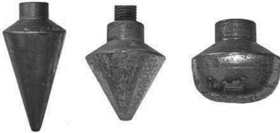
Figure 5. Cones made: a) C1 – 30°; b) C2 – 60°; c) C3 – hemisphere.
