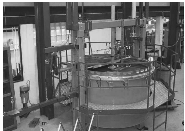
Figure 2. Test setup for cyclically long-term loaded monopiles.
