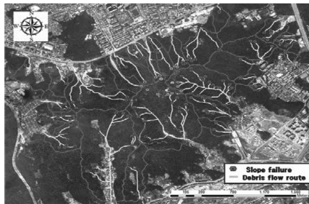
Figure 3. Locations of Slope Failures and Debris Flows around Umyeon Mountain in 2011
