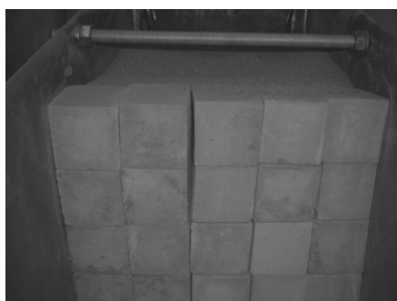
Figure 3. Model test showing concrete blocks partially rotated and wedged in against the sides of the test box.
