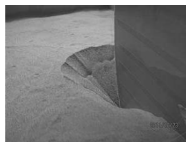
Figure 5. A close-up photo of the upstream inverse conical shape at H=36.78 cm (E0317)
