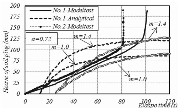
Figure 8 Predicted and measured heave vs. time curves
