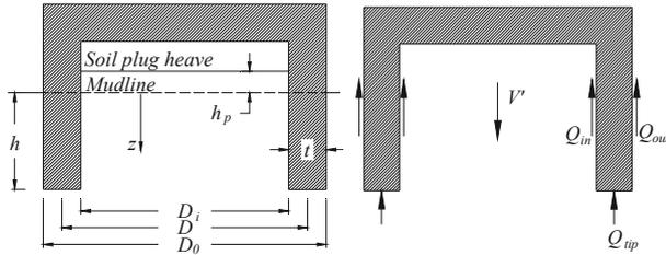
(a) Parameters definition (b) Free body diagram
