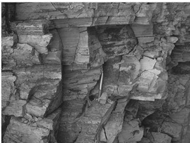
Figure 2. Stiff to hard silty clay layer to be cut and retained with anchored wall and surcharged with reinforced soil fill.
