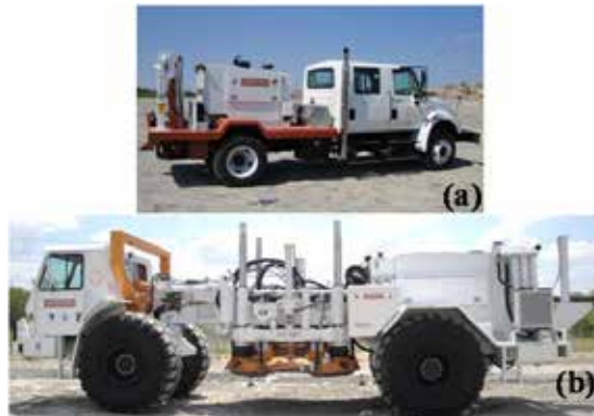
Figure 2: Photographs of large mobile shakers used to apply static and dynamic loads to the MSW: (a) Thumper and (b) T-Rex.
