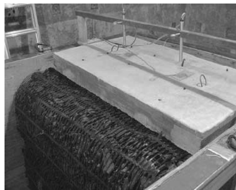
Figure 3. Constructed model MSE wall
