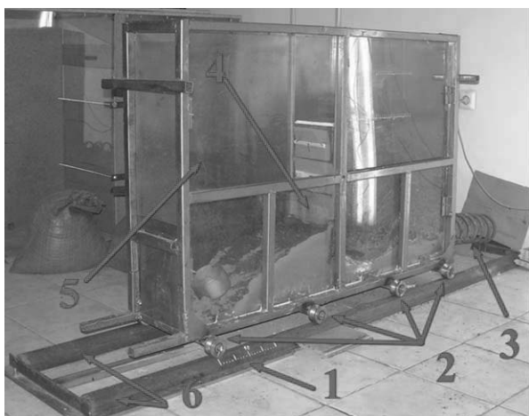
1- Scale of compression of a spring; 2 - Basic castors; 3 Spring; 4-Temporary partition in the middle of the stand; 5 - Transparent plexiglas; 6 - Directing rails.
