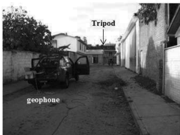
Figure 1. SASW instrumentation setup in one of the sites.
