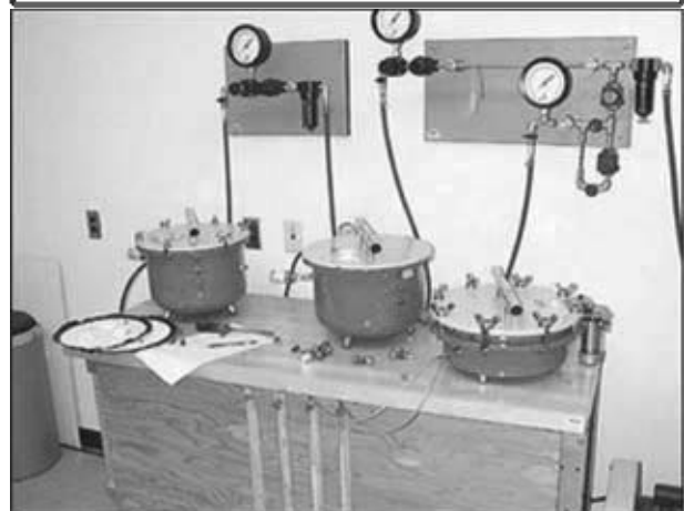
Figure 8. Pressure plate apparatus (from National Research Council Canada website).
