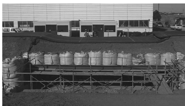
(1) Testing result after 550mm differential settlement
