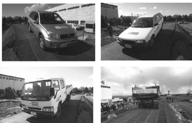
Photographs 8. Trafficability tests of Confined-Reinforced Earth
