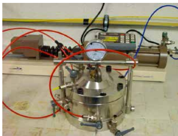
Figure 3. Suction controlled oedometer cell.
