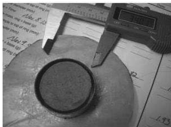
Figure 1. Digital micrometer used for the measurement of the diameter and thickness of shrinkage specimens.
