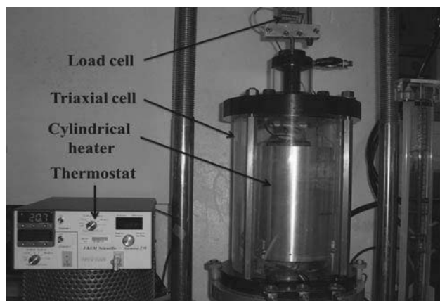
Figure 1. Suction and temperature controlled cyclic triaxial apparatus.
