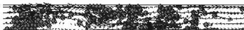
Figure 12. Unstable flow with formation of particles packs at initial c_v = 0.39 in 4mm wide channel with fluid flow velocity vectors around packs.
